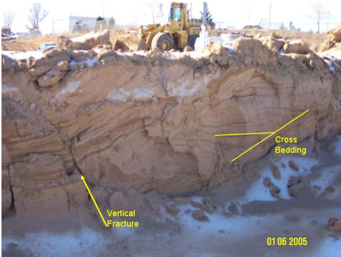
Figure 4. Cross Bedding and Vertical Fractures at Kern Center Pond
