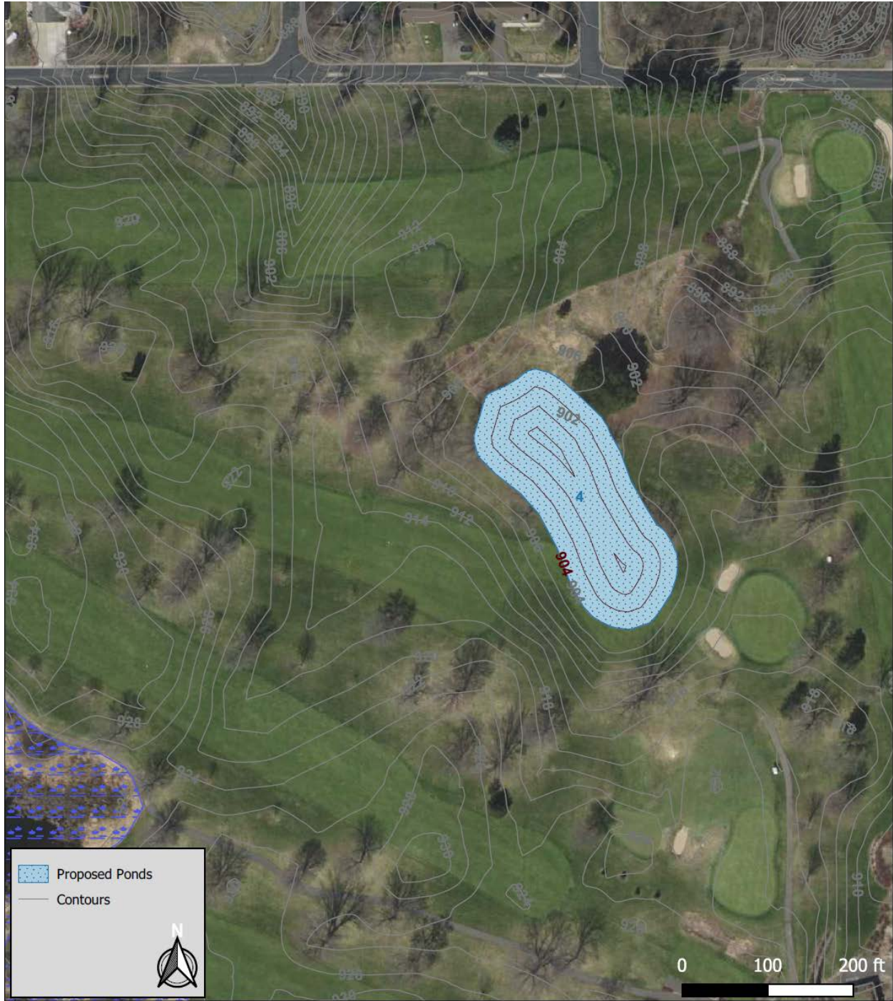
Figure 4 - Surface grading required for Pond 4
