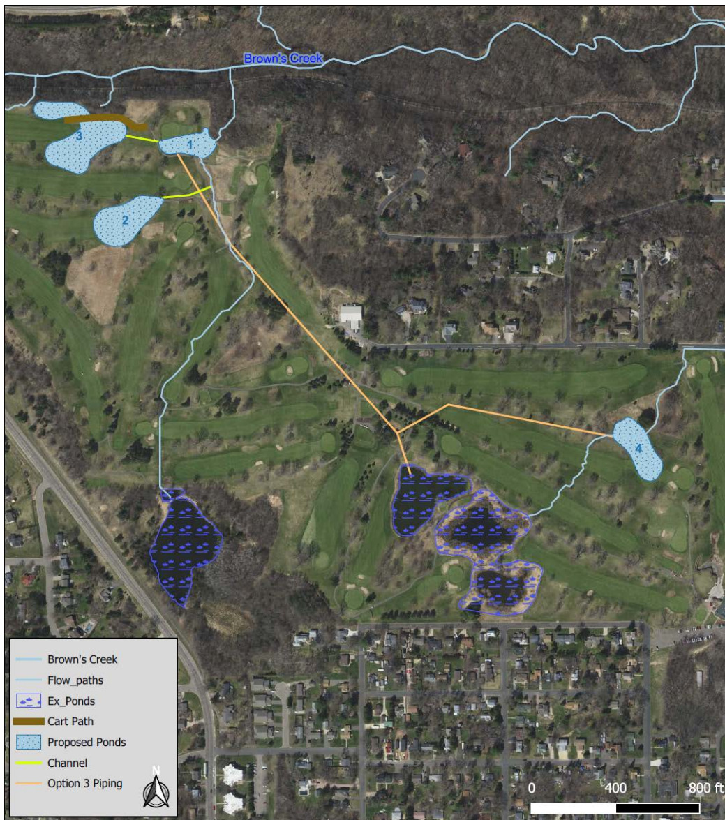
Figure 8 – Wetland storage combined with proposed stormwater ponds
