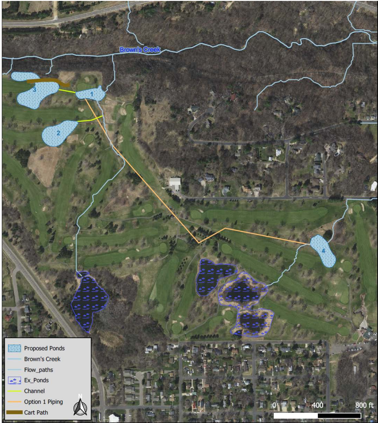
Figure 5 - Distribution Lines for Option 1 no cistern
