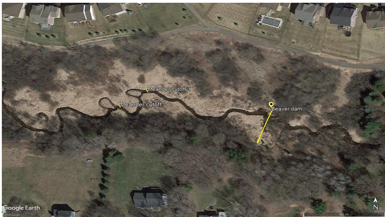
Figure 4. Brown's Creek on April 5, 2017 showing the locations of the meander cutoffs following the beaver dam failure.
