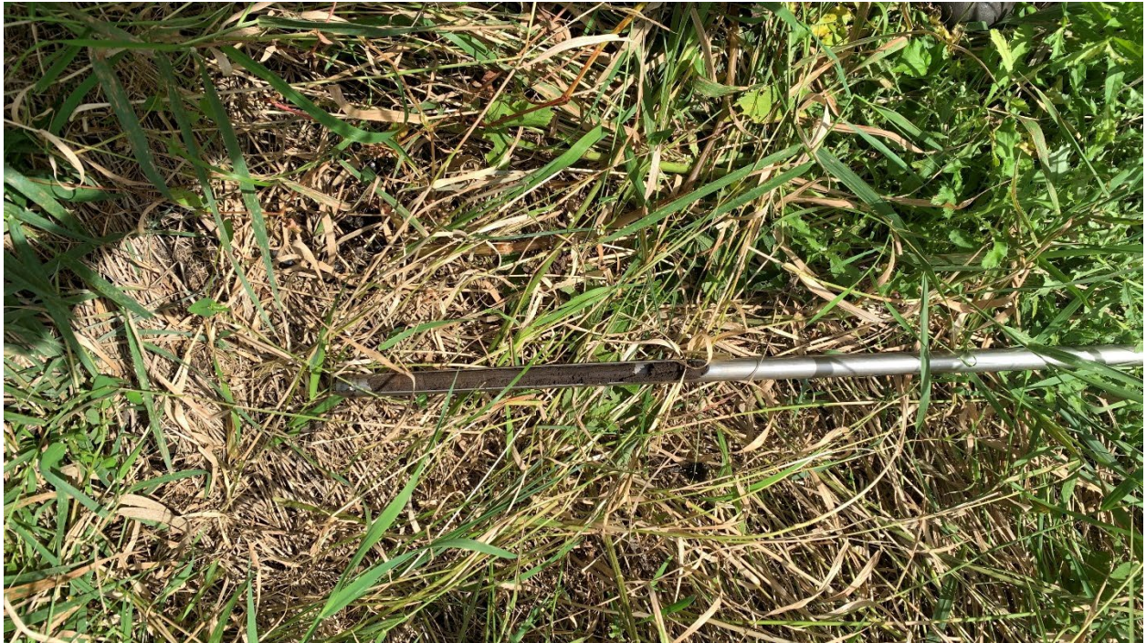
Figure 12. Soil probe from near center part of the project area. Iron staining near base of probe and soil saturated.
