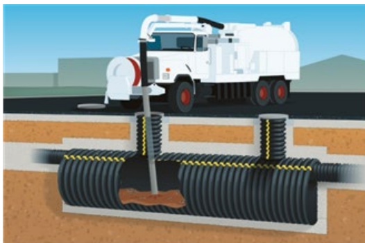
Figure 5. Maintenance of WQU
